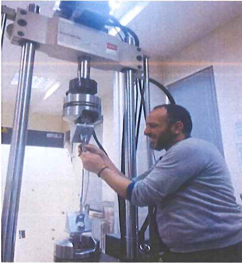
Pic.3 – Test Setup and Test Machine (647 Hydraulic Wedge Grip)
